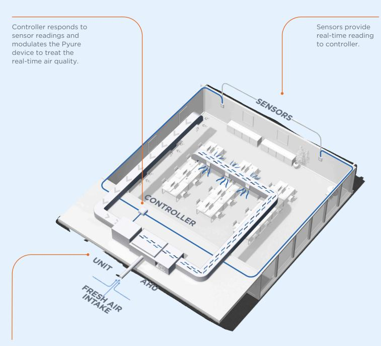
Hydroxyl unit works with single or multiple air handling systems.
